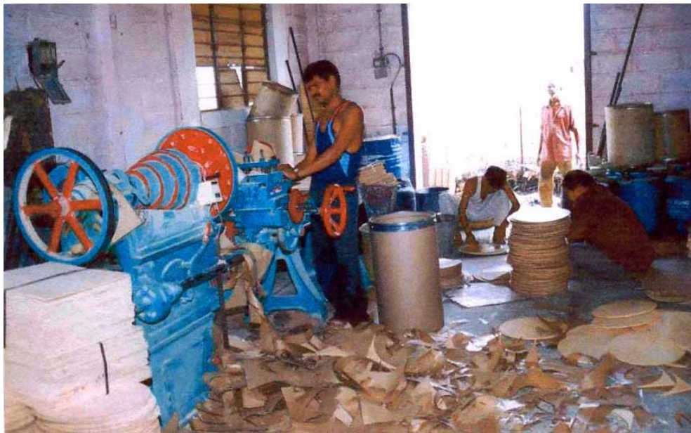
Circular cutting of lids for fibre drums
