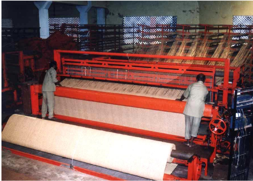
4m. Semi Automatic Loom
